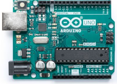
Figure 9: An Arduino Uno was used to gather sensor readings, actuate the motors and sample analog voltages.
