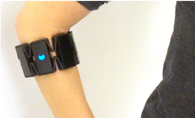
Figure 1. The Myo sensor bracelet used to measure gestures.
